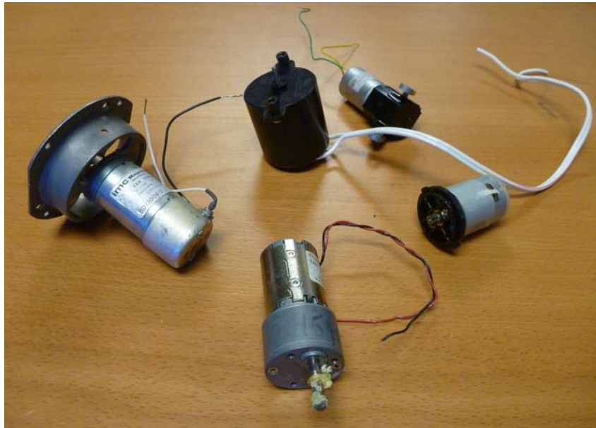
Figure 4.4: Slightly larger motors. These motors are around 3-4 inches long, and operate at voltages ranging from 9v to 24v. The motor in the front center has a gear head. This attachment (the dull gray part) is a gear reduction unit that slows the rotation down to around 20 RPM. The gear reduction also increases the torque dramatically. The motor on the left has a fan attached.
