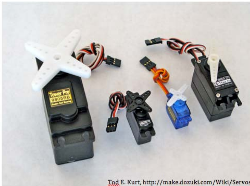
Figure 4.2: Servos come in a variety of sizes. Larger servos have more torque, but consume more power.
