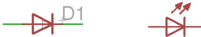
Figure 2.1: Schematic symbols for a general diode and a light emitting diode (LED).
