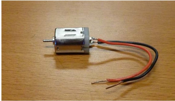
Figure 4.3: A tiny DC motor. A motor like this (approximately an inch long) typically spins very fast with a small voltage. This motor is rated at 5v.
