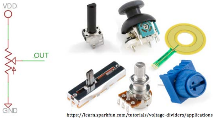
Figure 3.9: A standard potentiometer connection with the endpoints connected to VDD and GND, and the output being read from the wiper. Potentiometers come in a huge variety of shapes, sizes, and resistance values. Shown in the right of this figure are just a few different examples.
