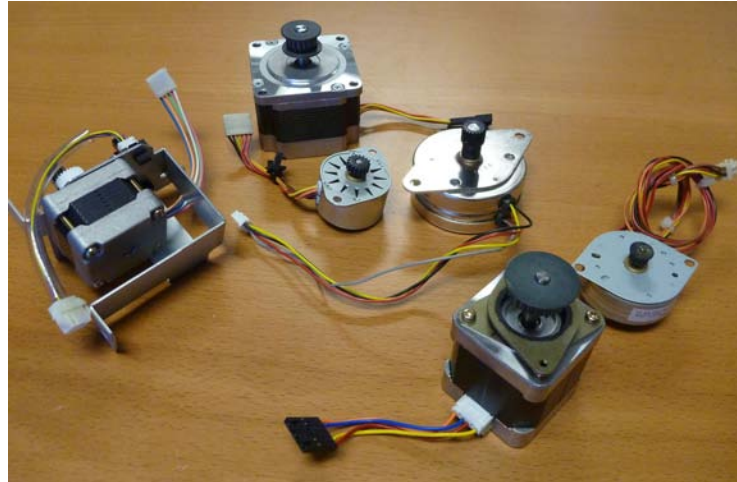
Figure 4.15: Some stepper motors in different sizes and types. Any steppers with four wires are bipolar steppers. Steppers with six wires are unipolar. These steppers include new motors and motors pulled from old equipment such as scanners. There is no standard color coding for control wires. A little exploring with an ohmmeter will help you figure out which ones are connected through a coil, and which are connected to different coils (i.e. not connected to each other).
