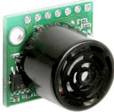
Figure 3.14: : Maxbotix sonar sensor. This sensor returns an analog voltage that varies as V_{dd}/512v per inch.
